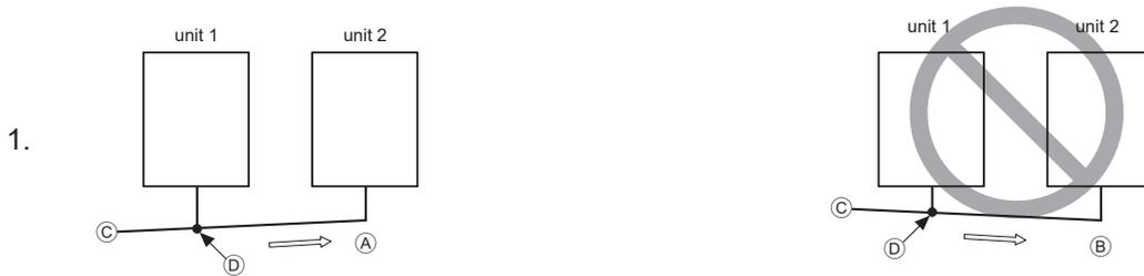
The NG example shows that oil accumulates because the units are installed on a reverse gradient while unit 1 is in operation, and unit 2 is stopped.
